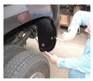
**Step 2:** Remove 2 factory metric bolts shown above. Points A & B
